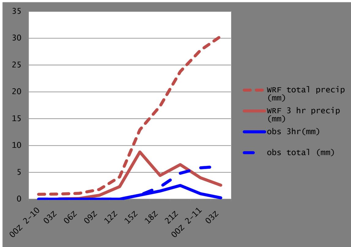
**Figure 2-2 WRF ARW simulation vs. observed precipitation for Anchorage Int'l Airport, February 10 -11, 2005.**
