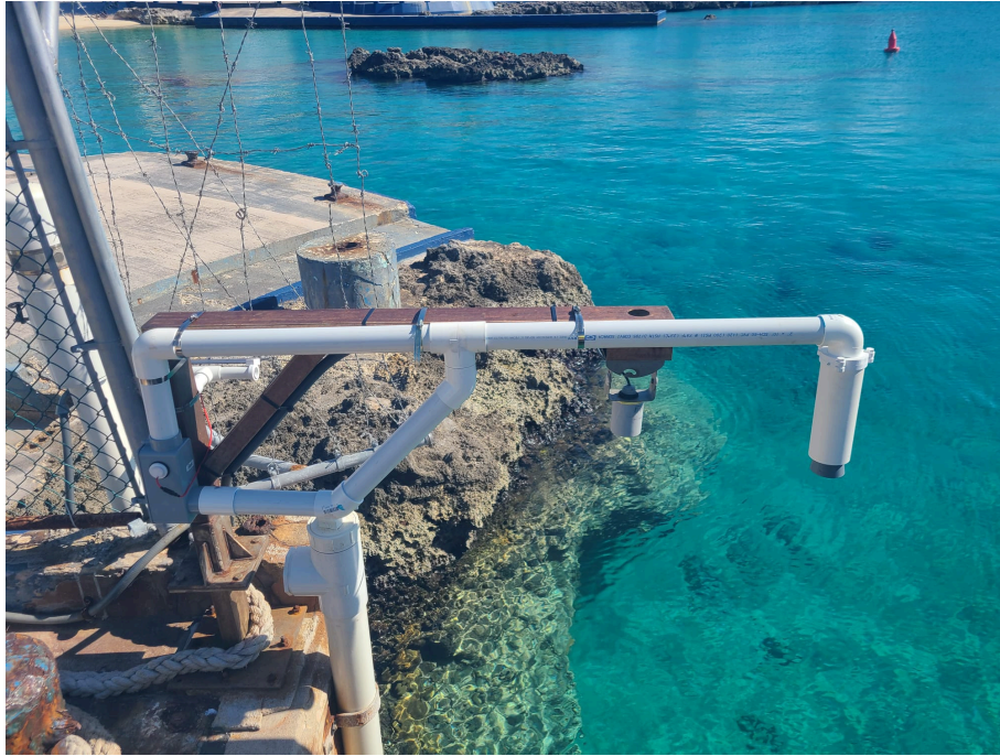
The storm surge sensor detects changes in water levels to provide early warning of inundation hazards.
