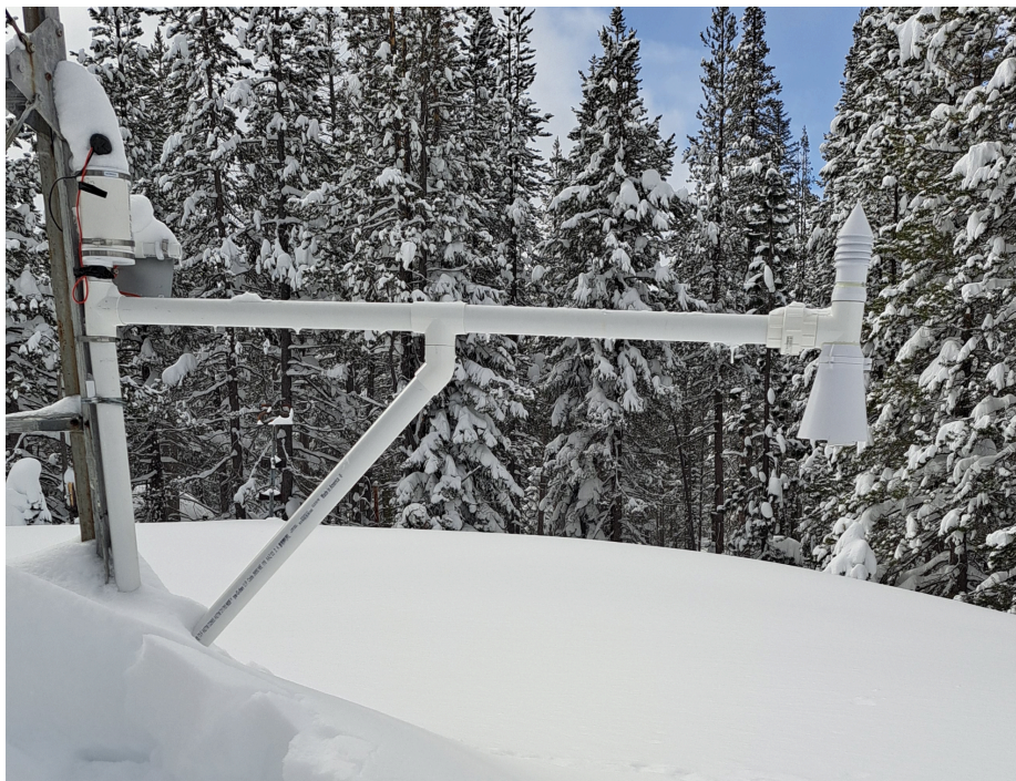
The snow depth sensor provides early detection of seasonal changes and snowmelt.
