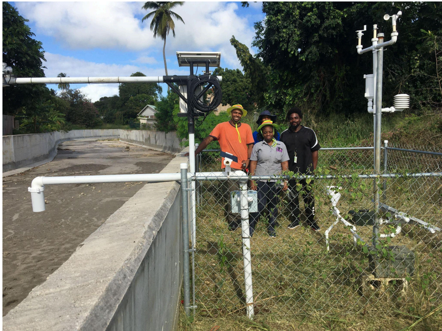
A 3D-PAWS stream gauge sensor at the Speightstown stormwater canal in Barbados next to the standard 3D-PAWS.
