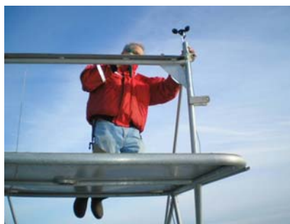
Figure 4. A WFO Juneau forecaster installs an anemometer on one of the vessels used to collect in situ data.
